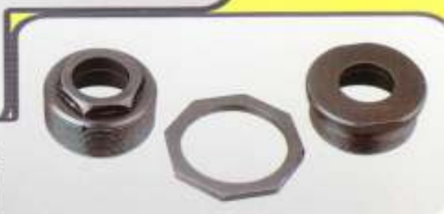
SE-502-A1 BB CUP WITH SEALED CARTRIDGE Fitted With Sealed Ball Retainers Octagonal Ring Thread : 34.8 X 24TPI 2P
