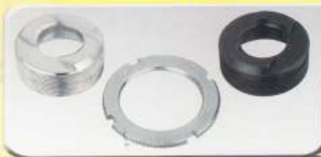
SE-502-C B.B. CUP PH TYPE Set of 3 Thread : 34.8mm X 24 TPI BSCY Rh/Lh Finish : BCP/2P/No Order
