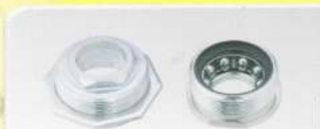
SE-502-A1 BB CUP WITH SEALED CARTRIDGE Fitted With Sealed Ball Retainers Octagonal Ring Thread : 34.8 X 24TPI 2P
